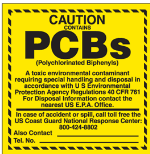
Figure 5: An example of PCB equipment labeling 36
